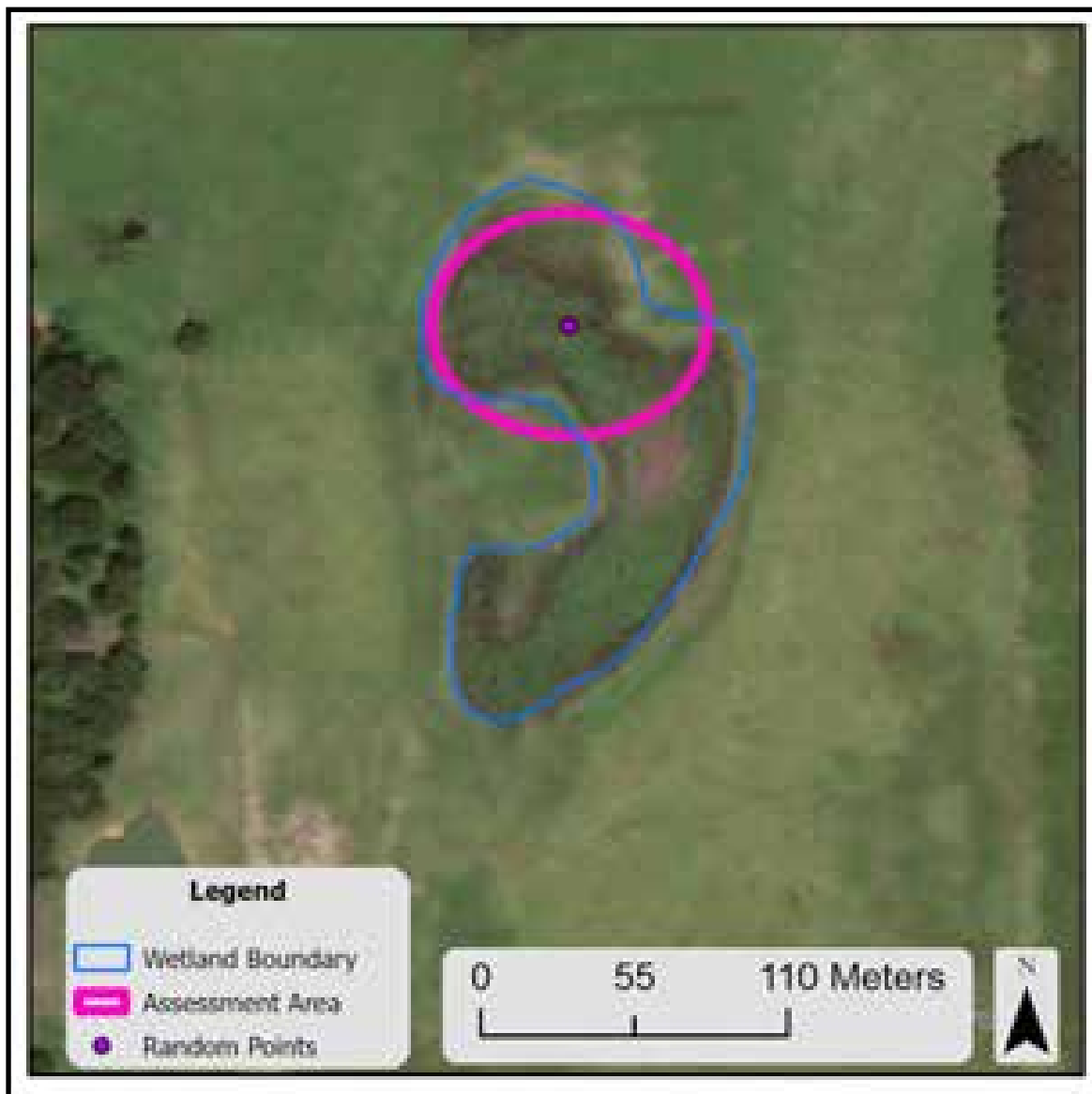
Fig 16. One hectare wetland. A random point was generated and a Standard AA was generated using the Create Random Point and Buffer tools in ArcGIS.
