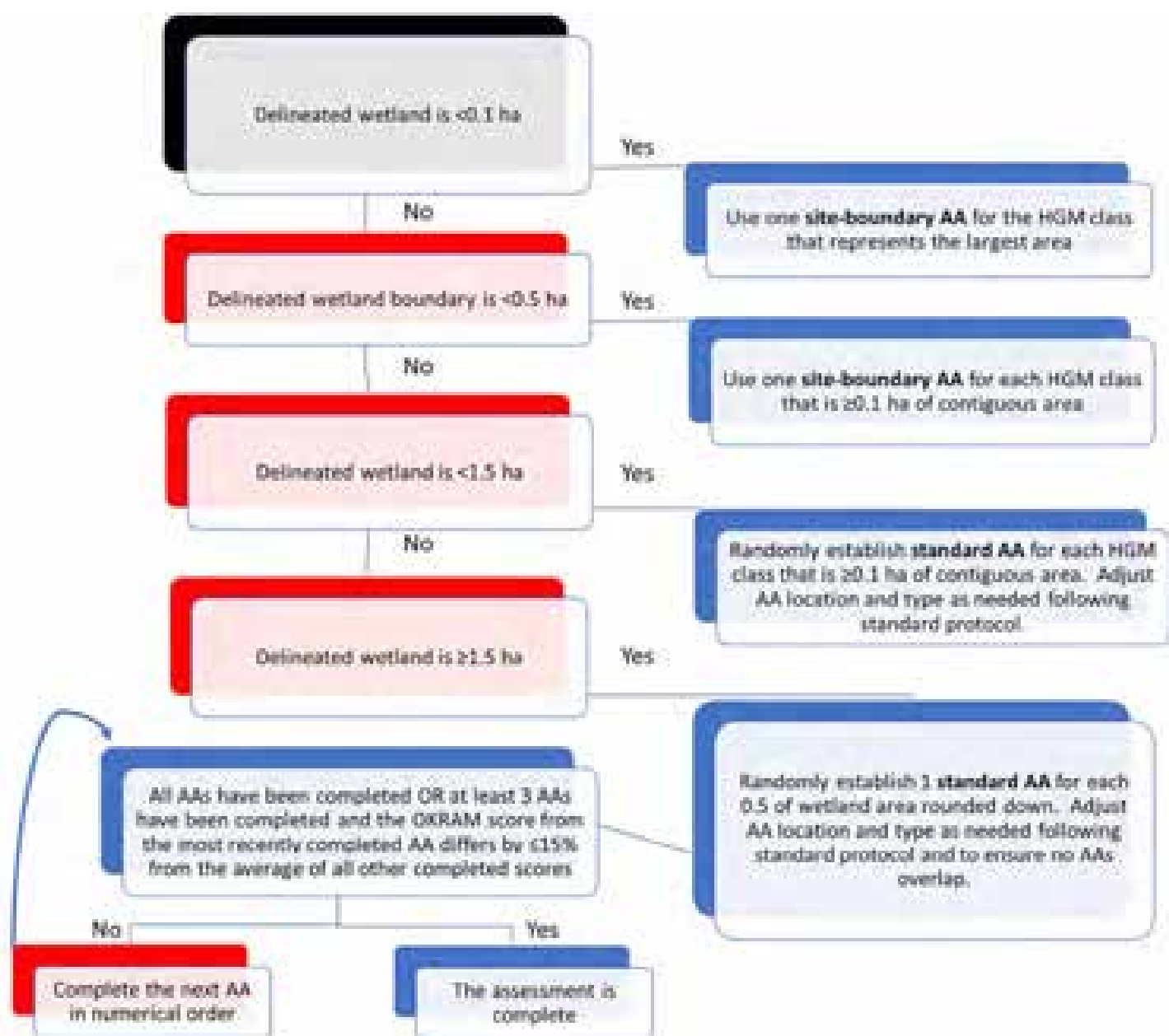
Fig 19. Flow chart for OKRAM AA creation for Site-Specific assessments of wetland condition . For pre- and post-restoration assessment replace all instances of the word “wetland” above with the words “project boundary”.
