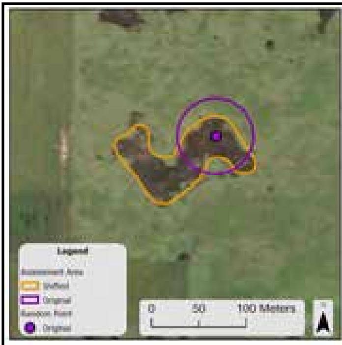
Fig 22. Step 2: Narrow wetland with an average 30 meter width, where a 40-m radius circular AA will not fit (top and bottom right). A 30-meter wide polygon, 166 meters long is created to retain a 0.5 ha. A polygon AA can be created that contains the original point, which minimizes the distance the point is moved (top right). Site boundary AA is used on a wetland that is smaller than 0.5 ha (bottom left).
